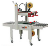
FXJ6050 Semi Automatic Carton Sealer 半自动封箱机 Conveyor speed/输送速度: 20m/min Max. Package size/最大包件尺寸: W500xH600mm Min. Package size/最小包件尺寸: W150xH120mm Width of tape/胶带宽度: 50, 60mm Power consumption/耗功率: 0.18KVA Machine size/机座尺寸: 1650x850x1330mm
