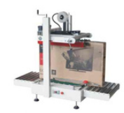
FXJ9050T Auto Carton Sealer 半自动封箱机 Conveyor speed/输送速度: 16m/min Max. Package size/最大包件尺寸: W500xH900mm Min. Package size/最小包件尺寸: W130xH110mm Width of tape/胶带宽度: 50, 60mm Power consumption/耗功率: 0.24KVA Machine size/机座尺寸: 830x840x1330mm
