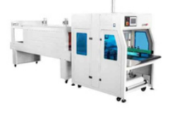
ST7040+BSE7040 Servo sealing and shrink packaging machine 伺服袖口密封收缩包装机 Sealing size/封口尺寸: W700*H400mm Working efficiency/工作效率: 0-25sets/min Power/功率: 30 KW, power supply: 3P/380V, Machine size/机身尺寸: L4000 * W1000 * H500mm
