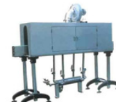
BSD1535ST Heat shrink wrapping machine 热收缩包装机 Fans power/风机功率: 0.37KW Steam pressure/蒸汽压力: 0.15-0.4Mpa Steam consumption/蒸汽流量: 20-100KG/H Tunnel size/收缩尺寸: 1800x150x350mm
