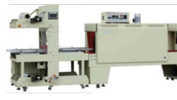
ST6040Z+BSE5045A Automatic cuff sealing machine 自动袖口式封切机 Seal size/封切尺寸: 550x430mm Working efficiency/工作效率: 8-12sets/min Power/功率: 30KW Sealing time/封口时间: 0.5-1.5s Tunnel size/收缩尺寸: L1500xW500xH450mm
