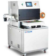
BTS400LV & BTS400LV/E Automatic Tray Sealer with Gas Flushing Inflation 气调密封包装机 Max. Tray Size/最大盒子尺寸: 490X330X50mm Zpsx 330X230X50mm or 4psx 230X150X50mm Max. Width of Film/最大膜宽: 300mm Max. Diameter of Film/最大膜管直径: 200mm Packing Speed/包装速度: 3 cycle/min. Pump Capacity/流量: 100m³ (BTS400LV) Options: Vacuum & Sealing (BTS400LV) Nitrogen Filling (BTS400LV, E) & Sealing Only (BTS400LV, E)
