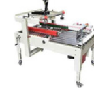
FXJ4030V (+Sealing Model) Carton Sealing Machine 自动封箱机(配套十字封胶) Power Supply/供给电源: 110V-220-240V/50-60Hz Power/功率: 240W Conveyor Speed/输送速度: 20m/min Max. Carton Size/最大纸箱尺寸: L550xW350xH400mm Min. Carton Size/最小纸箱尺寸: L200xW80xH90mm Width Of Tape/胶带宽度: 50mm
