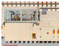
CE54030D High Speed Box Machine 高速开箱机 Suitable Cases/适用纸箱: L250-450mm W150-400mm H100-300mm Work speed/开箱速度: 20-40carton/min. Air Source/气源: > 850L/min, 0.4-0.8 Mpa Machine size/机器尺寸: L1100xW1250xH1740mm Air consuming/空气消耗量: 800L/min
