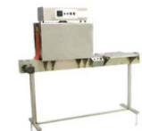
BSD11535 Heat shrink wrapping machine 热收缩包装机 Power/功率: 4KW Conveyor speed/输送速度: 0-4m/min Tunnel size/收缩尺寸: 700x150x350mm Conveyor loading/输送重量: 5KG Max
