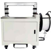
M23 Automatic Strapping Machine 全自动捆扎机 Strapping tension/捆扎力: 40-600N Adjustable Strapping speed/捆扎速度: 2.18Sec./Strap Strap width/捆扎带宽度: 9, 12, 15mm Arch size/捆扎尺寸: 800x600mm
