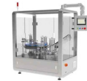
BZH50(VERTICAL Model) Automatic Cartoning Machine 自动装盒机 Power Supply/供电电压: 3\text{P } 220\text{V or } 380\text{V } 50\text{Hz} Main Motor Power/功率: 750\text{W} Working Speed/箱速: 40 \sim 50\text{cartons/min} Carton Size/适用箱尺寸: L65 \sim 220 \times W50 \sim 180 \times H15 \sim 80\text{mm} Air Source/气源: 0.6 \sim 0.8\text{Mpa } 450\text{l/min}
