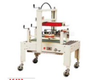
A5423 Semi Automatic Carton Sealer 半自动封箱机 Conveyor speed/输送速度: 20m/min Max. Package size/最大包件尺寸: W500xH500mm Min. Package size/最小包件尺寸: W150xH70mm Width of tape/胶带宽度: 50, 60mm Power consumption/耗功率: 0.18KVA Machine size/机座尺寸: 1100x900x1320mm
