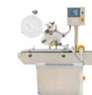
ALB210 Automatic Top Labeling Machine 自动顶部贴标机 Automatic Top Labeling Machine 标签宽度/Label width: A: 10-110mm C: 10-170mm 标签长度/Label length: 10-300mm 产品的宽度/Product width: A: 25-150mm C: 30-200mm 产品的高度/Product height: 10-250mm
