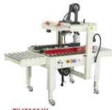
FXJ5060 III Semi Automatic Carton Sealer 半自动封箱机 Conveyor speed/输送速度: 20m/min Max. Package size/最大包件尺寸: W500xH500mm Min. Package size/最小包件尺寸: W150xH100mm Width of tape/胶带宽度: 50, 60mm Power consumption/耗功率: 0.18KVA Machine size/机座尺寸: 1860x850x1220mm
