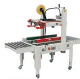
FXJ6050B Semi Automatic Carton Sealer 半自动封箱机 Conveyor speed/输送速度: 20m/min Max. Package size/最大包件尺寸: W500xH600mm Min. Package size/最小包件尺寸: W150xH120mm Width of tape/胶带宽度: 50, 60mm Power consumption/耗功率: 300W Machine size/机座尺寸: 1730x850x1380mm
