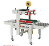
FXJ9050 I Semi Automatic Carton Sealer 半自动封箱机 Conveyor speed/输送速度: 20m/min Max. Package size/最大包件尺寸: W500xH500mm Min. Package size/最小包件尺寸: W150xH100mm Width of tape/胶带宽度: 50, 60mm Power consumption/耗功率: 0.18KVA Machine size/机座尺寸: 1660x850x1260mm
