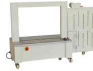
AP8060L Automatic Strapping Machine 全自动捆扎机 Strapping tension/捆扎力: 100-600N Adjustable Strapping speed/捆扎速度: 2.18Sec./Strap Strap width/捆扎带宽度: 9, 12, 15mm Arch size/捆扎尺寸: 800x600mm
