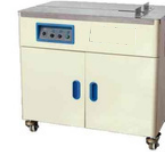
SM10H Semi-Automatic Strapping Machine 半自动捆扎机 Strapping tension/捆扎力: 40-400N Adjustable Strapping speed/捆扎速度: 0.535Sec./Strap Strap width/捆扎带宽度: 5-15mm Power consumption/耗用功率: 0.2KVA
