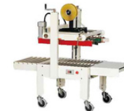
A5123 Semi Automatic Carton Sealer 半自动封箱机 Conveyor speed/输送速度: 20m/min Max. Package size/最大包件尺寸: W500xH600mm Min. Package size/最小包件尺寸: W100xH80mm Width of tape/胶带宽度: 50, 60mm Power consumption/耗功率: 0.18KVA Machine size/机座尺寸: 1580x740x1330mm
