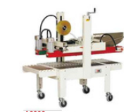
A5232 Semi Automatic Carton Sealer 半自动封箱机 Conveyor speed/输送速度: 20m/min Max. Package size/最大包件尺寸: 1600xW500xH600mm Min. Package size/最小包件尺寸: 1200xW150xH100mm Width of tape/胶带宽度: 50, 60mm Power consumption/耗功率: 0.18KVA Machine size/机座尺寸: 2000x850x1220mm
