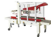
FX-AT5050 Automatic Flap-fold & Bottom Sealer 全自动折盖封底机 Conveyor Speed/输送速度: 16m/min Max. Package Size/最大包件尺寸: W500xH500mm Min. Package Size/最小包件尺寸: W120xH120mm Power Supply/供给电源: 110V-220-240V/50-60Hz Power Consumption/功率: 240W Width Of Tape/胶带宽度: 60mm Machine Size/机器尺寸: 1780x950x1400mm Machine Weight/机器重量: 240kg
