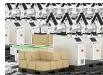
BPK-M550 cooperative palletizing robot 协作码垛机器人 palletizing speed/码垛速度: 3 \sim 8\text{times/min} applicable pallet/适用托盘: 1800 \times 1200 \times 150 \sim 200\text{mm} power/电压: 220\text{V } 50\text{Hz} air source/气压: 0.5 \sim 0.8\text{kg/cm}^2
