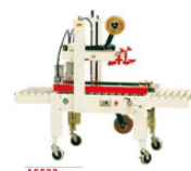
A5523 Semi Automatic Carton Sealer 半自动封箱机 Conveyor speed/输送速度: 20m/min Max. Package size/最大包件尺寸: W500xH580mm Min. Package size/最小包件尺寸: W100xH100mm Width of tape/胶带宽度: 50, 60mm Power consumption/耗功率: 0.18KVA Machine size/机座尺寸: 1740x850x1320mm
