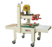
A5223 Semi Automatic Carton Sealer 半自动封箱机 Conveyor speed/输送速度: 20m/min Max. Package size/最大包件尺寸: W500xH800mm Min. Package size/最小包件尺寸: W100xH80mm Width of tape/胶带宽度: 50, 60mm Power consumption/耗功率: 0.18KVA Machine size/机座尺寸: 1550x820x1320mm
