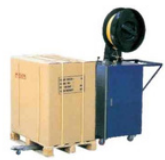
DBA130A Automatic Strapping Machine 半自动捆扎机 Strapping tension/捆扎力: 100-600N Adjustable Strapping speed/捆扎速度: 2.05Sec./Strap Strap width/捆扎带宽度: 9-15mm Chute size/出料尺寸: L1000mm Power consumption/耗用功率: 0.5KVA
