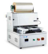
BTS400T/E & BTS400T/S Automatic Tray Sealer with Gas Flushing Inflation 气调密封包装机 Max. Tray Size/最大盒子尺寸: 330X200X50mm or 2psx 220X150X50mm Max. Width of Film/最大膜宽: 300mm Max. Diameter of Film/最大膜管直径: 200mm Packing Speed/包装速度: 3 cycle/min. Options: Nitrogen Filling (BTS400T/E) Sealing Only (BTS400T/S)
