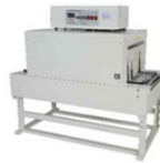
BSD350/400/450 Heat shrink wrapping machine 热收缩包装机 Heater power/加热功率: 6.5KW(Adjustable) BSD350 6.5KW(Adjustable) BSD400 8.0KW(Adjustable) BSD450 Conveyor speed/输送速度: 0-10m/min Tunnel size/收缩尺寸: 830x350x150mm BSD350 830x400x200mm BSD400 830x450x250mm BSD450
