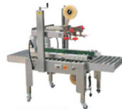
FXJ6050/A55235 Semi Automatic Carton Sealer 半自动封箱机 Conveyor speed/输送速度: 20m/min Max. Package size/最大包件尺寸: W500xH800mm Min. Package size/最小包件尺寸: W100xH100mm Width of tape/胶带宽度: 50, 60mm Power consumption/耗功率: 0.18KVA Machine size/机座尺寸: 1740x850x1330mm
