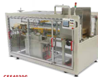
CE54030G High Speed Box Machine 高速开箱机 Suitable Cases/适用纸箱: L250-450mm W150-400mm H100-300mm Work speed/开箱速度: 20-40carton/min. Air Source/气源: > 850L/min, 0.4-0.8 Mpa Machine size/机器尺寸: L1120xW1250xH1740mm Air consuming/空气消耗量: 800L/min
