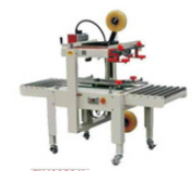
FXJ9050 II Semi Automatic Carton Sealer 半自动封箱机 Conveyor speed/输送速度: 20m/min Max. Package size/最大包件尺寸: W500xH500mm Min. Package size/最小包件尺寸: W150xH120mm Width of tape/胶带宽度: 50, 60mm Power consumption/耗功率: 0.18KVA Machine size/机座尺寸: 1650x850x1230mm
