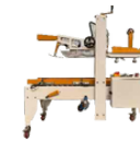
FX-AT5050L Automatic Flap-fold & Bottom Sealer 全自动折盖封底机 Work speed/封箱速度: 16m/min Max. Carton size/最大包件尺寸: L1100xW460xH1000mm Min. Carton size/最小包件尺寸: L300xW150xH200mm Width Of Tape/胶带宽度: 60mm Machine Size/机器尺寸: 3120x960x2040mm
