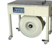
SM10T Semi-Automatic Strapping Machine 半自动捆扎机 Strapping tension/捆扎力: 40-400N Adjustable Strapping speed/捆扎速度: 0.535Sec./Strap Strap width/捆扎带宽度: 5-15mm Power consumption/耗用功率: 0.2KVA
